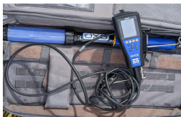
Figure 2: technical device for collecting data on water quality.
