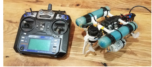
WW-03 utilizes an stick-type controller
