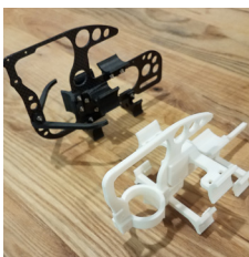
Redesign efforts successfully reduced the overall ROV height by 20% (2019-top left).
