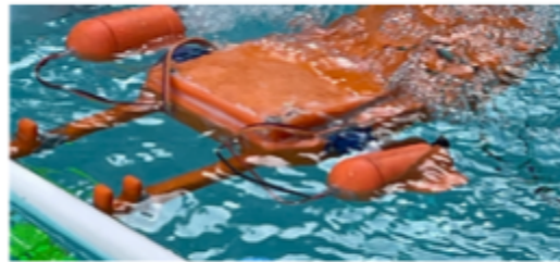
ROV positively buoyant without weights
