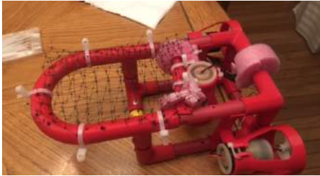
(Figure D) ROV while netting was being added, demonstrating the position of the motors and netting figuration.
