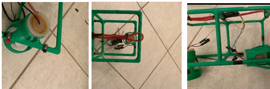
Figure 3: Ballast placement (left), tether placement (middle), motor placement (right).
