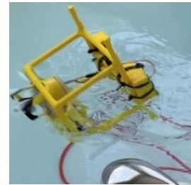
Figure 7: The short ROV frame in water-testing
