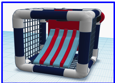
1st ROV Design: Neptune PVC frame with a scoop lined with magnetic strips
