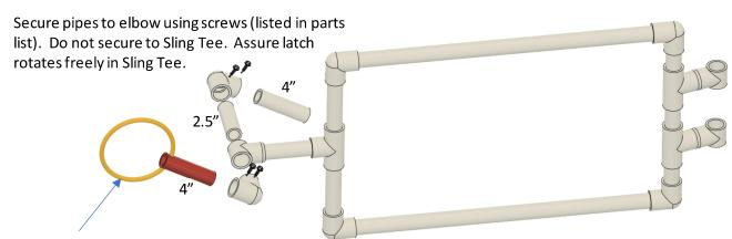
12" Long Polypropylene rope. Fasten ends using cable ties or suitable means.
