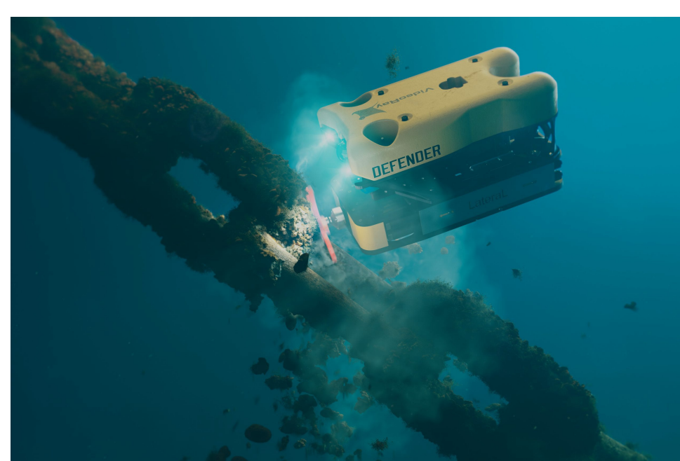
Figure 3. ROV cleaning underwater infrastructure (Lateral, 2025).
