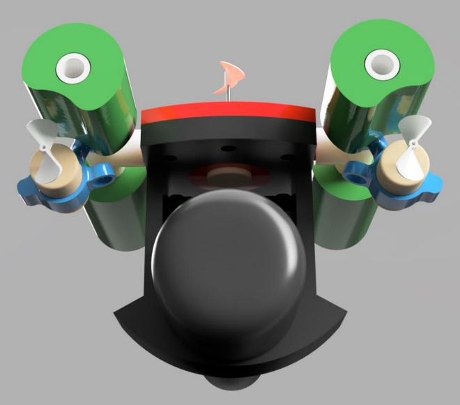
This is the Bathymetric SeaPerch ROV that we designed. The red piece on top would be 3D printed. It would hold the SONAR system below it, the vertical thruster in the middle, and the flotation and horizontal thrusters on either side.
