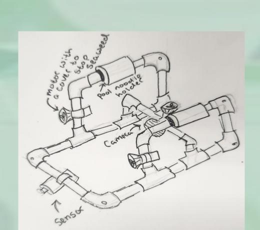
Then, we imagined and planned how it would look and the materials we would need to get there. We took our ROV design from this year and added a camera and the PFAS sensor. Additionally, we included a special motor holder with a cover around the propeller to prevent seaweed and other debris from tangling in the motor.
