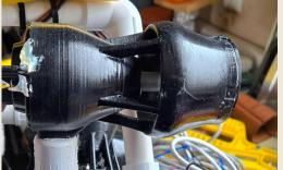
Thrusters are 500 gallons per hour (gph) bilge pump cartridges. Each fitted with 3D printed kort nozzles and removable screens, or "motor covers"
