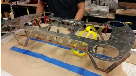
The main hull is made of several sections to allow for future modifications and ease of maintenance. The center section of the main hull is comprised of a ½” aluminum tube that has been faced off so that industry standard what tight connectors can be mounted. It acts much like a spine for all the thrusters and external sensors and instruments. On each end of the main hull
