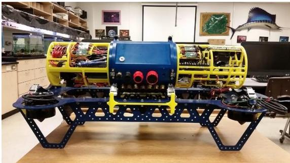
are removable polycarbonate tubing bordered by an aluminum ring on one side and a thermal exchange endcap on one tube and a acrylic done on the other tube. The
