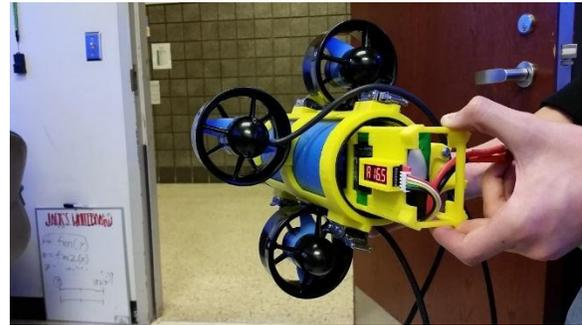
The same type of setup is used for the pneumatics module and the DVL module. The DVL is slightly different in that it has an aluminum fixture on one end so that it could accommodate the DVL head that needs to be in a 90° differential in relationship to the polycarbonate tube that houses the electronics.
