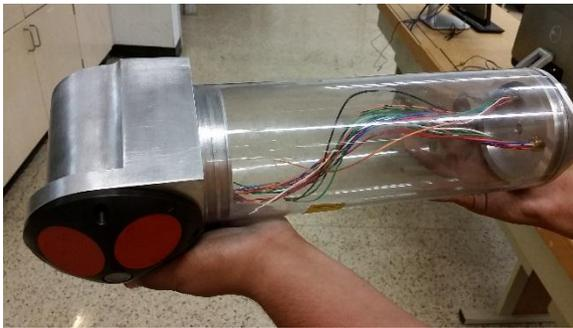
KVH DSP-1750 single axis Fiber Optic Gyro (FOG) The DSP-1750 FOG provides an ultra stable angle sensor that is capable keeping drift below 0.1 deg/hr (one sigma) when properly calibrated under optimal conditions. The gyro has enough stability to accurately measure the rotation rate of the
