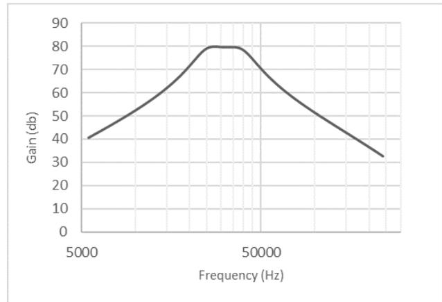
Fig. 11: SPICE simulation of amplifier frequency response
