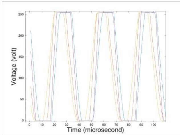
Fig. 12: Sampled Pinger pulse over time
