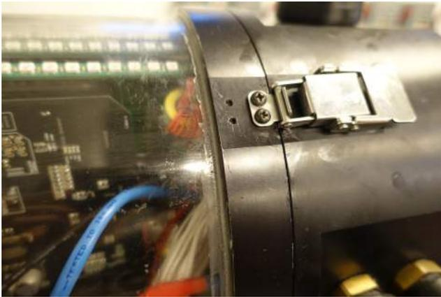
Fig. 5: Aluminum collar fastened to endcap
