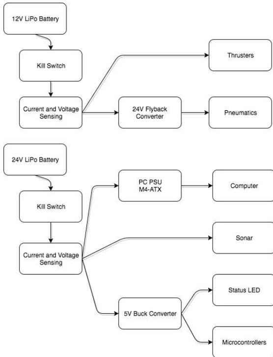
Fig. 9: Power system diagram
