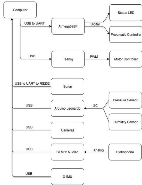
Fig. 10: Input/Output system diagram
