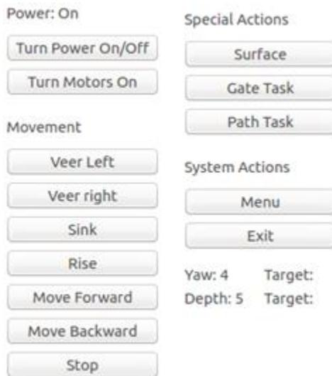
Fig 9. Users can trigger commands and check the IMU through the GUI
